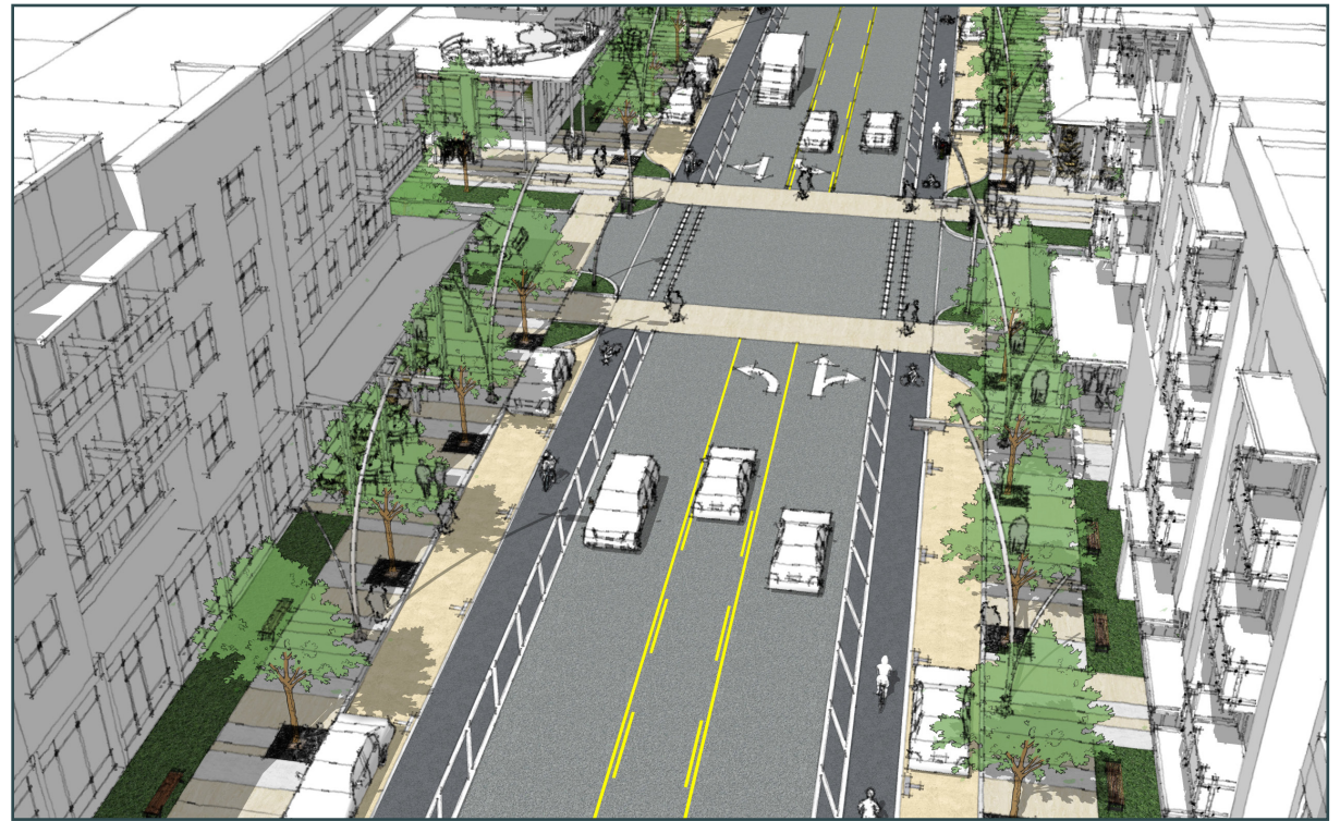
Figure 1.8 Preferred Option 3-Lane Cross-Section from Pleasant Run Rd. to Heath Creek
