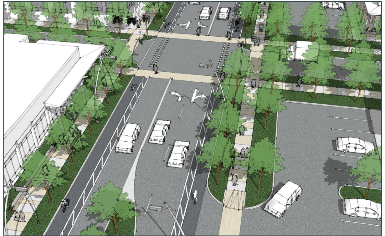
Figure 1.10 Preferred Option 2-Lane Cross-Section from Heath Creek to Belt Line Rd.
